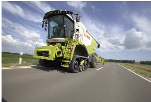
LEXION 750 with TERRA TRAC - its unsurpassed road speed is 40 km/h.
