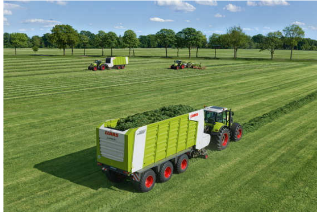
CARGOS with 30.5 inch tyres and weight indicator
