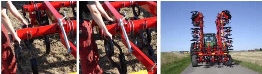
Through an ingenious telescopic solution, the largest models can be adjusted so that their transport height is less than 4 m.
