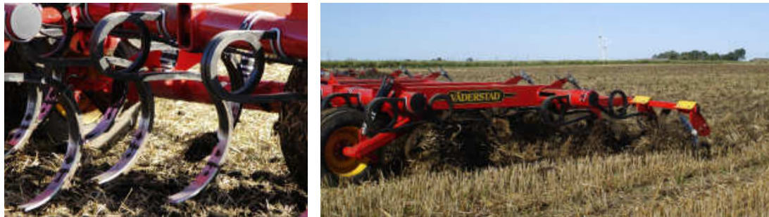
Four rows of vibrating tines with the MixIn shin do an impressive job on stubble.
