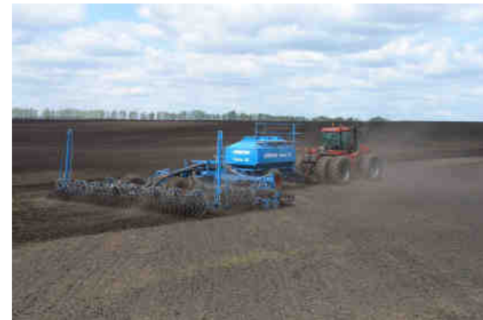
Drill combination with pneumatic seed trailer Jantar compact disc harrow in the Russian Black Earth region
